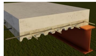
Steel beam with composite slab, 3D drawing rendered by LumenRT
