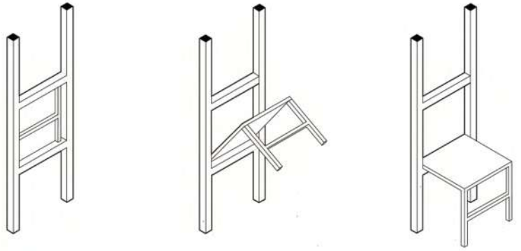
Foldable chair and table mechanism that is integrated in to the pavillion wall. Make the interior space flexible and easy to manage.
