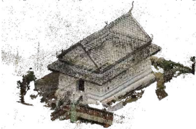
1. Point cloud generated by photogrammetry software (Agisoft Photoscan)
