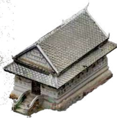
2. Polygonal mesh processed from pointcloud
