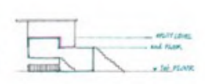
OVERLAPPED Each floor shares space together, second-floor use roof of the first floor that is a different height of a ceiling
