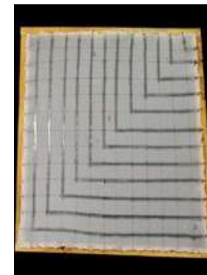
5. Applying resin with the help of brush in the geometric pattern.
