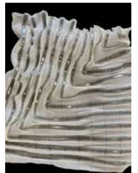
6. Letting the resin to dry and then pulling out the fabric from frame
