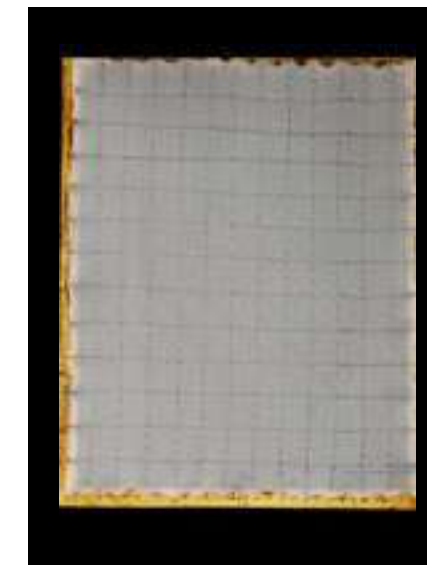
3. Fixing the fabric with frame with the help of nails
