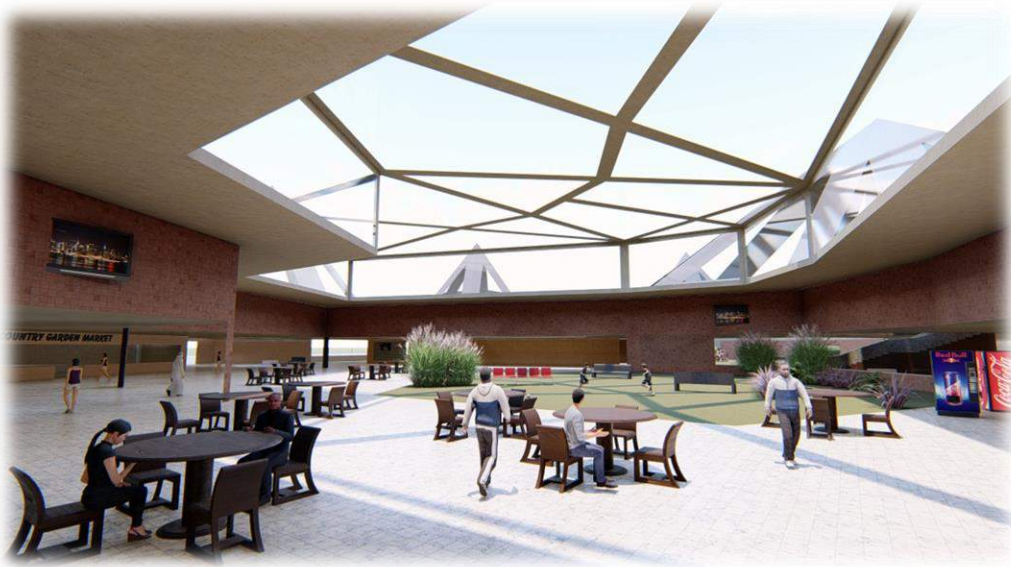
Skylight effect in the interior. Skylight opening towards north to let in the diffused light
