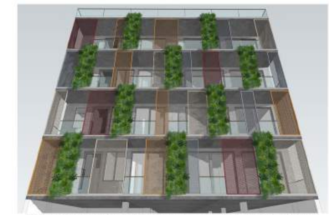
The panels painted in different hues stand-out in the otherwise restrained concrete façade. The screen with green wall in the facade cuts off the glare and reduces heat gain in the summer months.
