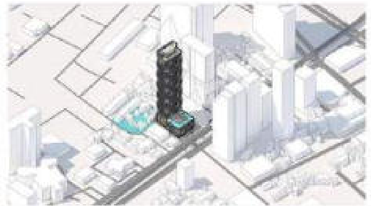
The final design pushes the building rise until it almost touches the 2H line and makes the room benefit as double volume
