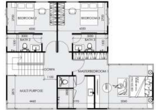
TYPE 2 GROUND AREA 82.40 SQ.M 2ND AREA 100.00 SQ.M TOTAL 182.40 SQ.M 2nd FLOOR PLAN 0 2.5 5 7.5 SCALE 1:100@A3
