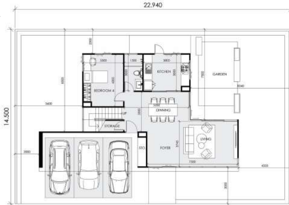
GROUND FLOOR PLAN 0 2.5 5 7.5 SCALE 1:100@A3 LAND AREA 332.63 SQ.M
