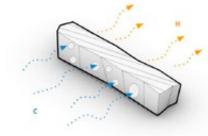
In this stage, finding the strategy to achieve cross ventilation in terms of openings will be our topic for design. The wind pressure seems to be related to the velocity and indicable to locate the position on the building facade in order to bring the wind in.
