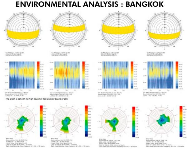
First, The Sun path of Bangkok showing the angle that directly from Southern upto perpendicular angle in Summer correspondes to the dry bulb temperature of Bangkok where the hottest period happening during April to Jun.
