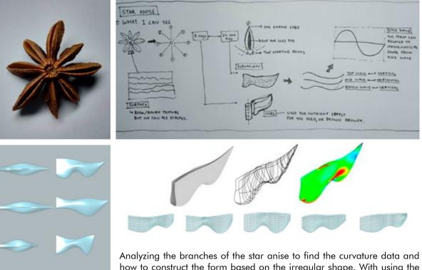
Analyzing the branches of the star anise to find the curvature data and how to construct the form based on the irregular shape. With using the methematics, the project end up using sine waves to variate the different modules and developed further into human scale installation.
