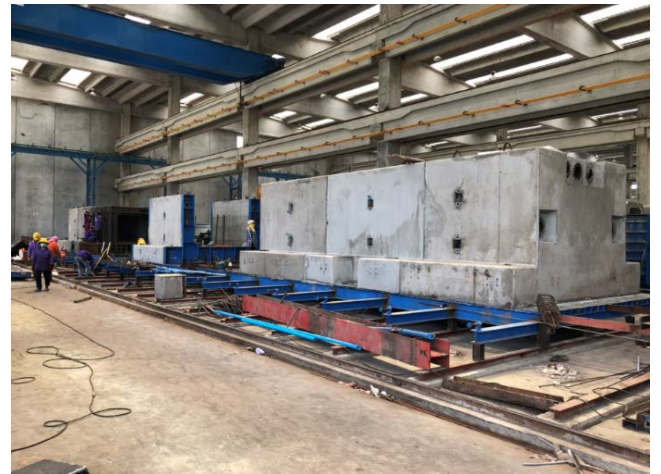
Precast segment in factory
