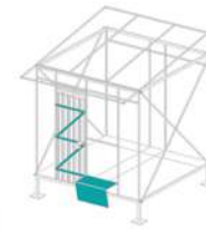
Fixing the door sheet and window cum bench to the framework
