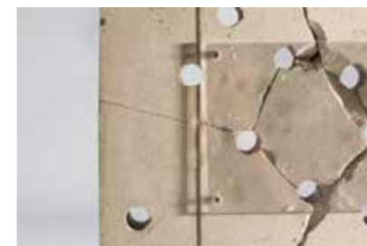
Added scaffoldings used to mark drill hole positions and glass panels to trap water inside drilled holes. Expansion of water as ice is form fissure the concrete material in a curated manner.
