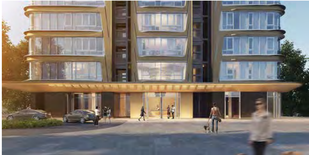
01 CANOPY REQUIRED FOR DROP OFF AND ENTRANCE 02 BASE GEOMETRY FOLLOWING TOWER FIN DESIGN 03 BUTTERFLY SKYLIGHT ALLOWING LIGHT INSIDE
