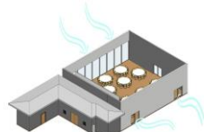
ISOMETRIC DRAWING SHOWS THE CROSS VENTILATION
