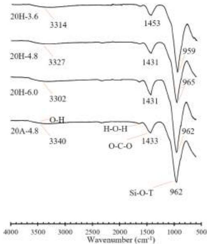
Fig. 7. figFTIR results for geopolymers made with RHA.
