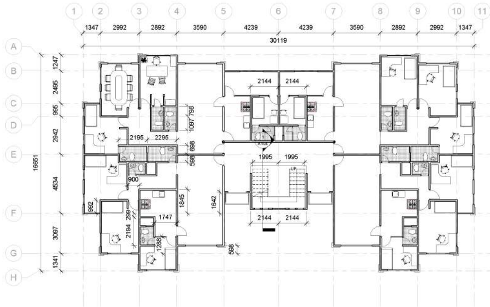
① 1st Floor Plan 1:100
