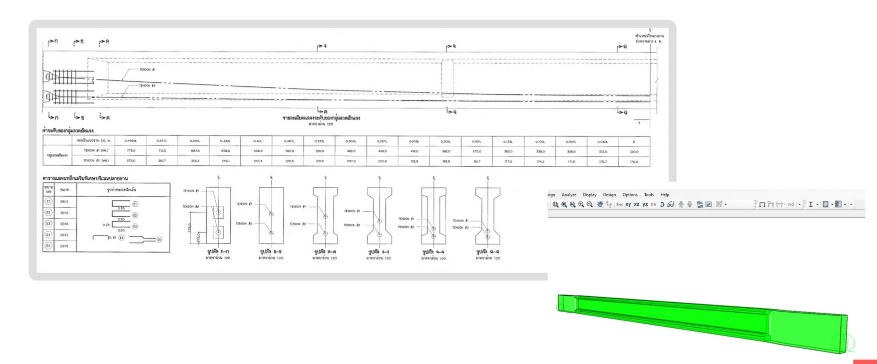
6. Calculate the prestressed concrete bridge girder forces during lifting and transportation. To determine the percentage of prestressed wire that should be pulled and how much early-strength concrete must be used to avoid damage to the prestressed concrete beams. and calculation of elongation of prestressed wire in post-tension.
