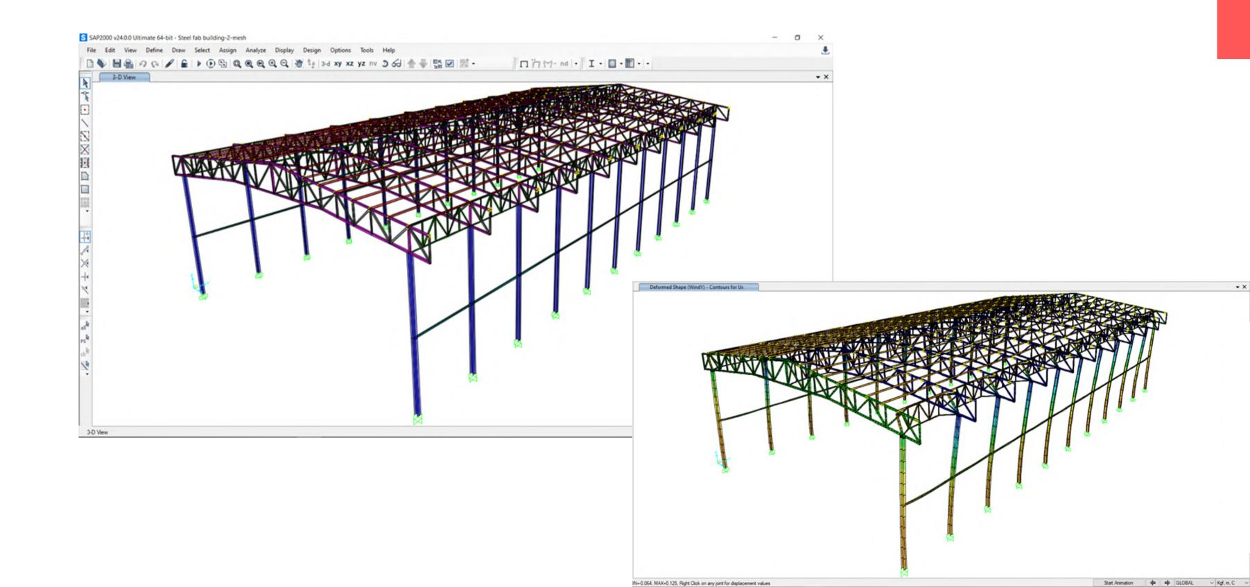
2. Design tower can support a load of 350 tons for lifting Expressway By using the SAP2000 Program.
