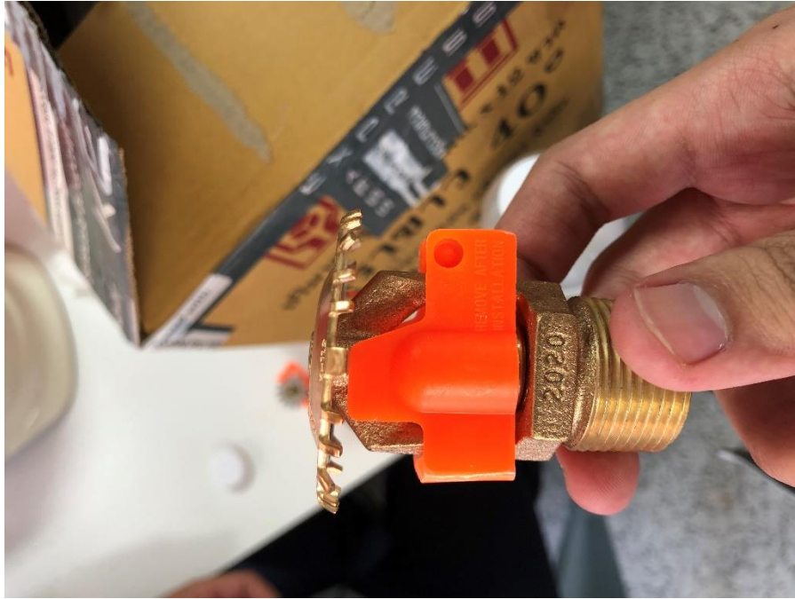
FIG.9 Sprinkler K11.2 EC type at Yellow Wood 6 New Warehouse
